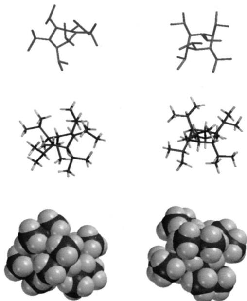
**Fig. 1.** All equatorial and all axial trans-1,2,3,4,5,6-hexa-isopropylcyclohexane depicted in tube (hydrogens hidden) model, in tube (hydrogens shown) model and in space-filled model.
