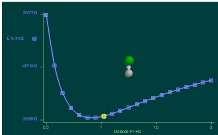
**Fig. 1** Screen shot from a video showing the change in potential energy as a function of the distance between an H and F atom.
