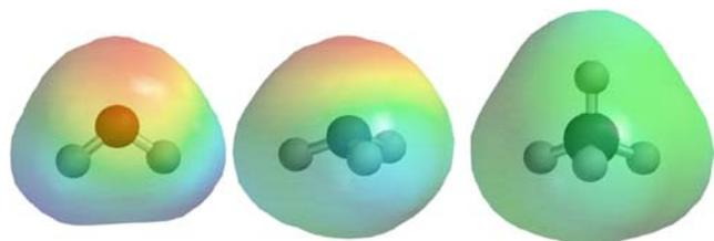
**Fig. 2** Electrostatic potential maps of H<sub>2</sub>O, NH<sub>3</sub> and CH<sub>4</sub>. These maps are used to discuss the consequence of electronegativity on electron distribution and the influence of molecular shape on molecular polarity.
